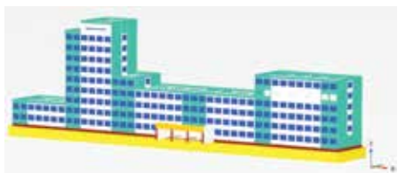
3-rasm. Seysmik to'siqli model.
